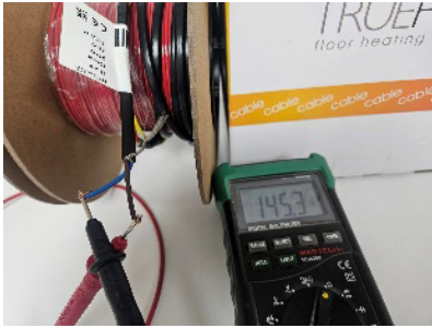
5. Measure resistance (1st time) (See section 8 for full details)
